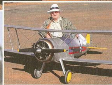
Winner of the Special Achievement award, Clive Butler competed with his 100-inch-span Gloster Gladiator in the Masters class. Powered by a 215cc Moki 5-cylinder gas 4-stroke radial engine, the big biplane spins a 32x18 prop. Construction is conventional plywood, balsa and spruce and the covering is SRTex fabric.
